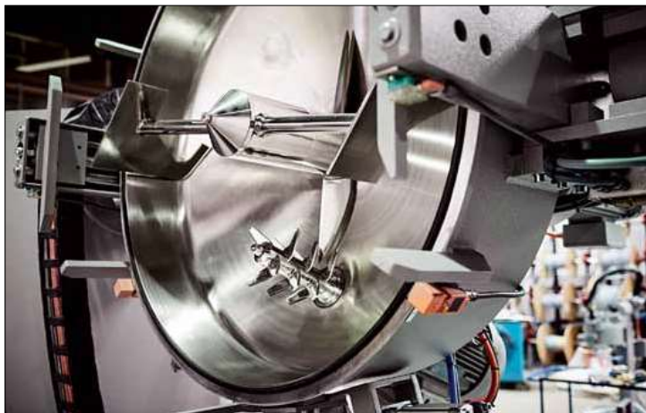
The MIXACO Multitool™ is an example of the thoughtful further development of the container mixer; reduced cleaning times and higher throughput are just two of the major benefits of using lower temperatures during mixing.
