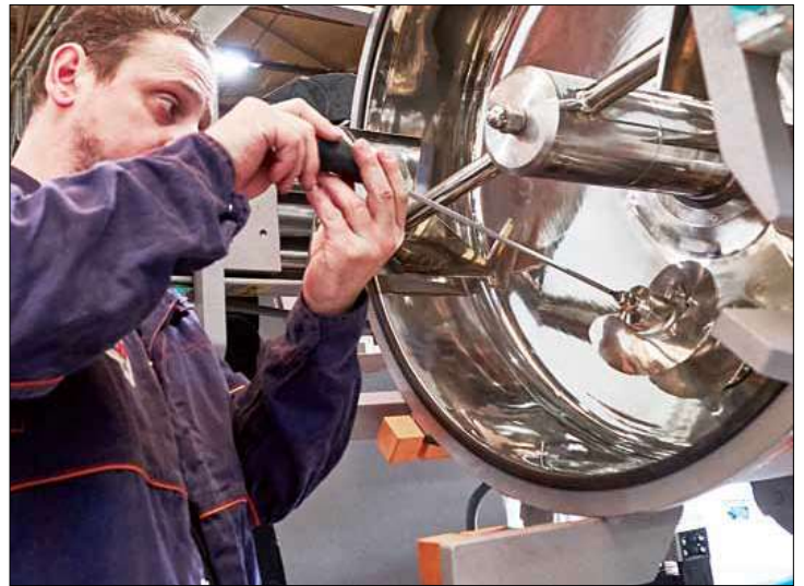
Mixing tools can be changed quickly as needed or when changing recipes; this means that the mixer is ready for the next batch after only a short space of time.
